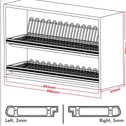
Size Adjustment Packing 3mm, 5mm & 8mm Size Adjustment Possible
